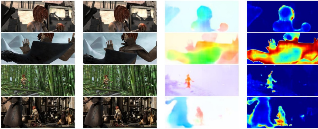
Figure 3: Examples of (a), (b) input images, (c) predicted flows, (d) predicted variances of FlowNetU on Sintel Clean.
